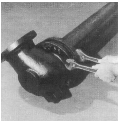
2. Remove all 6 Shoe Bolt Nuts.
